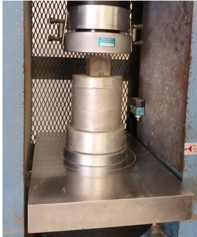
Figure 2. Compressive strength testing
